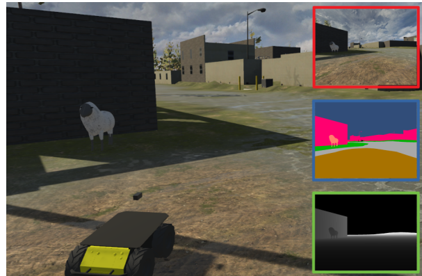
Fig. 1: A robot autonomously explores an unknown environment using an RGBD sensor and a semantic segmentation algorithm.
