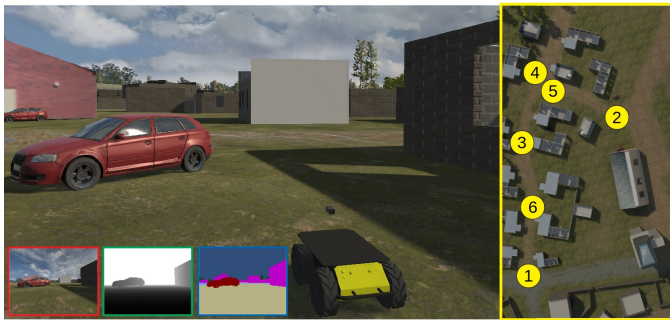
Fig. 6: Simulation environment for multi-robot distributed active mapping: A Husky robot receiving RGB, depth, semantic segmentation images. A top-down view of the simulated environment, where the numbered circles show the starting positions of six robots is shown on the right.
