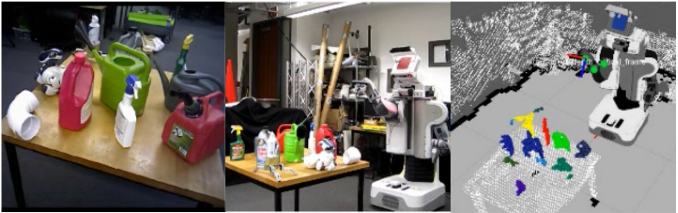
Fig. 7. Example of the experimental setup (left), which contains two instances of the object of interest (Handlebottle). A PR2 robot with an Asus Xtion RGB-D camera attached to the right wrist (middle) employs the NVP approach for active object classification and pose estimation. In the robot's understanding of the scene (right), the object which is currently under evaluation is colored yellow. Once the system makes a decision about an object, it is colored green if it is of interest, i.e., in \mathcal{I} , and red otherwise. Hypothesis H(0^\circ) (Handlebottle with yaw 0^\circ ) was chosen correctly for the green object. See the attached video or http://www.seas.upenn.edu/~atanasov/vid/Atanasov_ActiveObjectDetection_TRO14.mp4 for more details.
