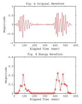
Figure 2. (A). ASD waveform after DWT and (B) the energy index profile.
