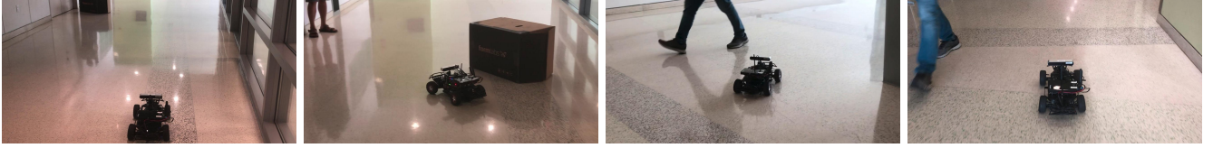
Fig. 4: Third person views of the autonomous Racecar robot navigating in an unknown environment with moving obstacles.
