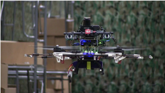
FIGURE 1 Our robot configuration showing the platform with stereo cameras and a nodding lidar
