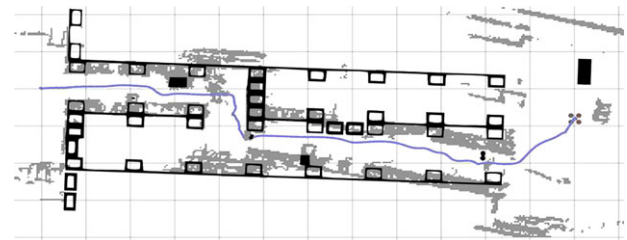
FIGURE 26 One of our runs for the aisle change with 90° transition task. In black, we show the actual obstacle course layout. The small filled black objects along the aisles are short obstacles that the robot could fly over. The gray regions are the projection of map created by the robot onto the 2D plane. The robot starts near the opening on the left and has to reach the target represented by the black rectangle on the right. Each grid cell is 5 m \times 5 m
