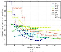
Fig. 7: (a). Mug, bottle, jar, bowl, glass, used for real robot experiments. (b). Experiment setup. (c). Real robot results. Distance to true class vs. number of poses, for baseline (dashed) and tree policy (solid). Dots and crosses show hits and misses. Each curve is an object.
