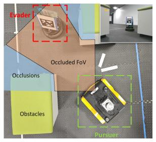
Fig. 1: A mobile *pursuer* aims to keep a mobile *evader* within its field of view despite occlusions and without colliding with obstacles. The inset shows the evader in the pursuer's camera view.
