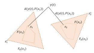
Fig. 2: Illustration of the proof that the visibility CBF is Lipschitz continuous in a 2D environment where the pursuer and evader states are positions and orientations. The triangles show the pursuer's unoccluded FoV, while the dashed polygons inside show the occluded FoV. The distances to the points  $\mathbf{z}_1$  and  $\mathbf{z}_2$  from  $\mathbf{y}(t)$  define the visibility CBF at  $\mathbf{x}_1$  and  $\mathbf{x}_2$ , respectively.
