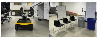
Fig. 6: Actual setup for 'S'-shape (left) and a section of long cluttered path (right). On the left, the pursuer navigates through rows of desks. The evader can be seen in the background to the right of the pursuer. On the right, the pursuer navigates through an aisle and turns two corners in an 'S-shape'.
