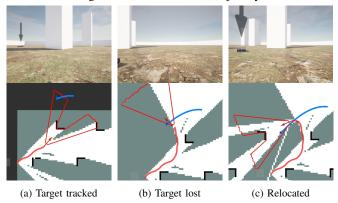
Fig. 4: Top: Snapshots from pursuer's view along its trajectory. Bottom: The red and blue curves denote the pursuer and evader trajectories, respectively. (a) The instance when the target is first observed by the pursuer; (b) The pursuer loses the evader around a corner; (c) The pursuer relocates the evader after turning the corner.
