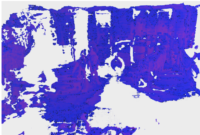
Fig. 9: Reconstruction of the Cow and Lady dataset. Red hues indicate lower TSDF uncertainty.
